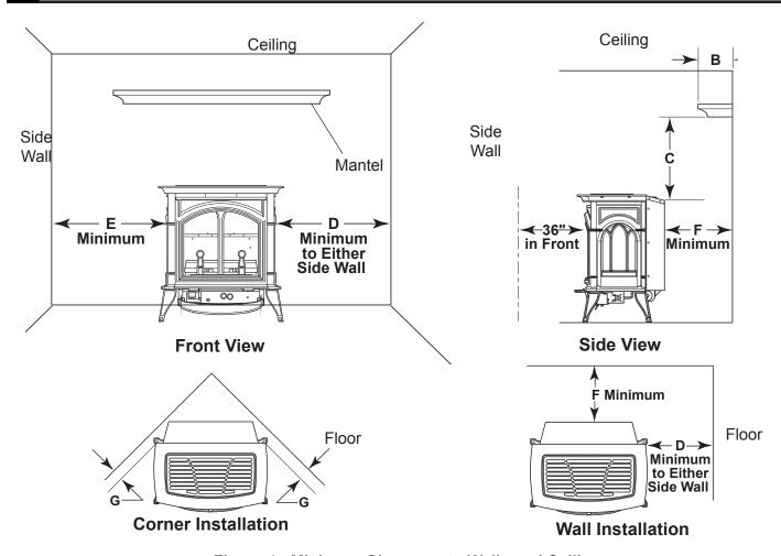
Figure 4 - Minimum Clearance to Walls and Ceiling
